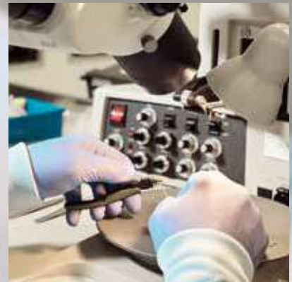
7154TC Carbide Insert Cutters suitable for tip cutting hard wire catheters and stents.
