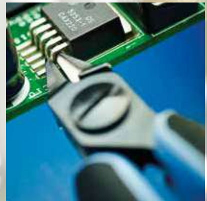
RX 8148 Ultra-Flush® diagonal cutter with tapered and relieved head is ideal for use in confined spaces and for rework.
