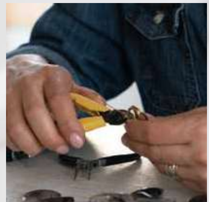
8141 cutters provide Flush cuts on bead wire and precious metals.
