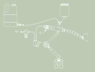
**b.** Setup for finely dispersed droplets
