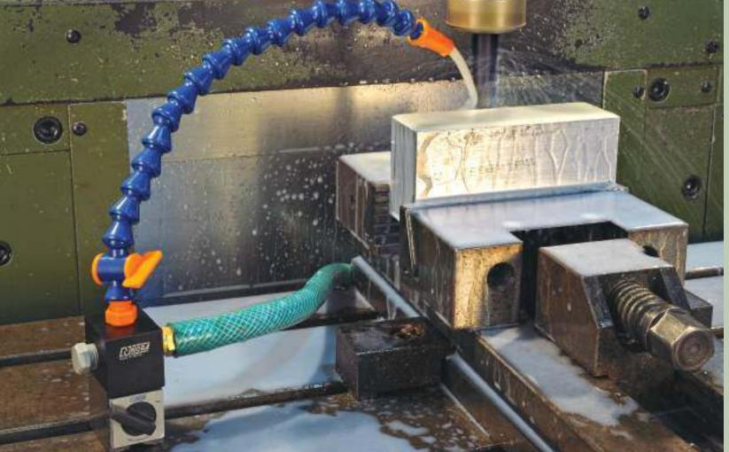
**NOGACOOL** consists of a manifold & Loc-Line<sup>®</sup> flexible hose with a nozzle on top and a valve at the bottom, assembled on the powerful on/off Popeye magnet.
